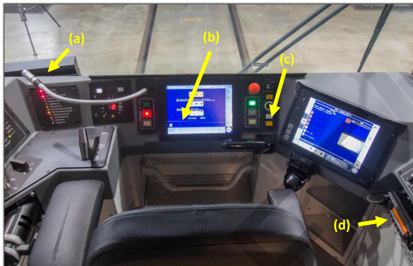
Figure 9. Photograph of inside the operating cab of Series 2 LRV with arrows pointing at (a) Microphone, (b) Live PA button location on TOD screen, (c) PTT button for intercom, and (d) LRV onboard radio. Source: LRV Operator Training Manual
